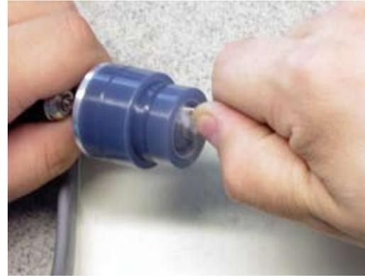
The filewax blanks are supplied in two versions: as cylinders with a 10 mm center hole or as full blocks. Due to the handy size and good accessibility of the wax blanks high quality parts can be done with a perfect surface finish.
