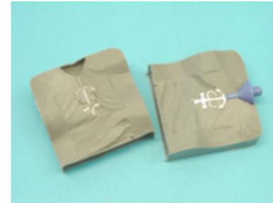
the mold is cut in halves.
