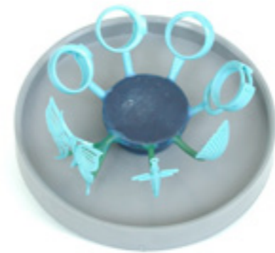
The finished pattern may be sprued alone or together with other parts for casting.
